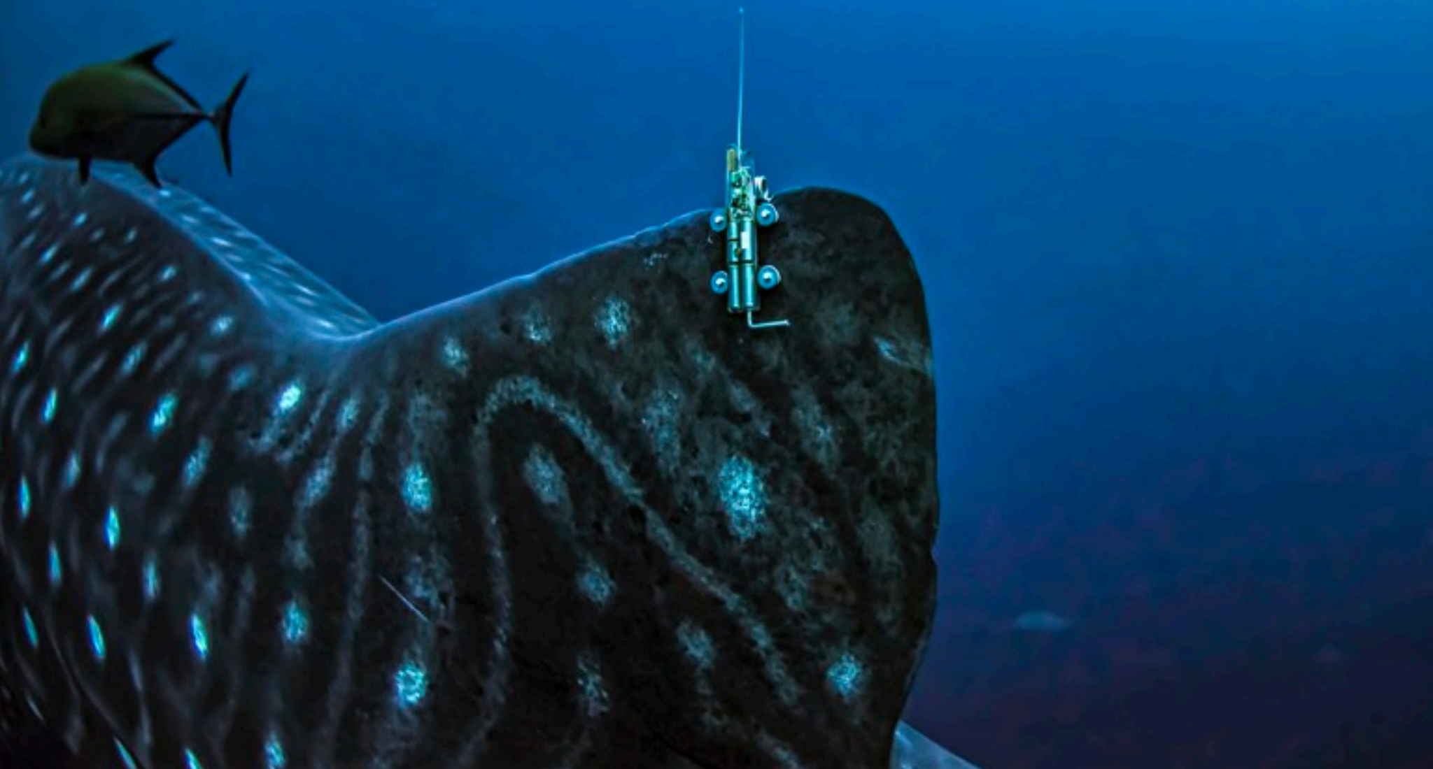
Figure 5: The SPLASH10 - 346B fin-mount tags sit high on the dorsal fin just fore of the apex. This ensures a strong position that will maximise transmissions and reduce risk of removal or loss. Photo © Jenny Waack, 2020
