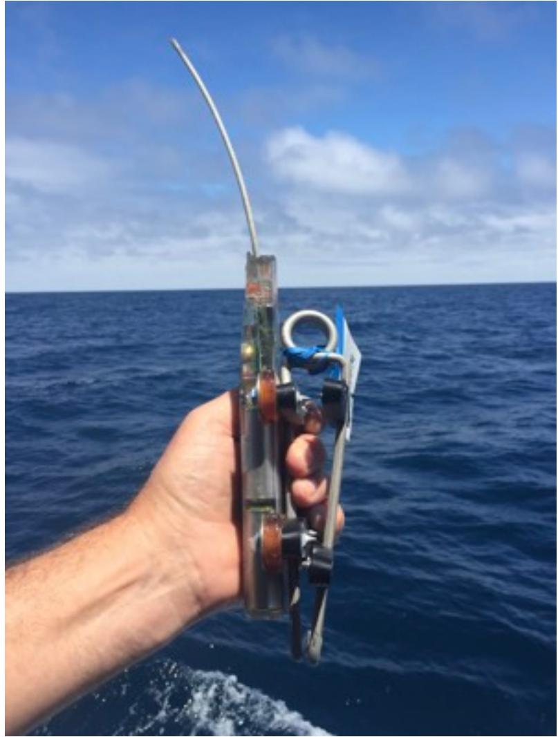
Figure 6: Tags mounted on fin clamps with nylon pads - SPLASH10-346B (Photos ©Sofia M Green, 2020)
