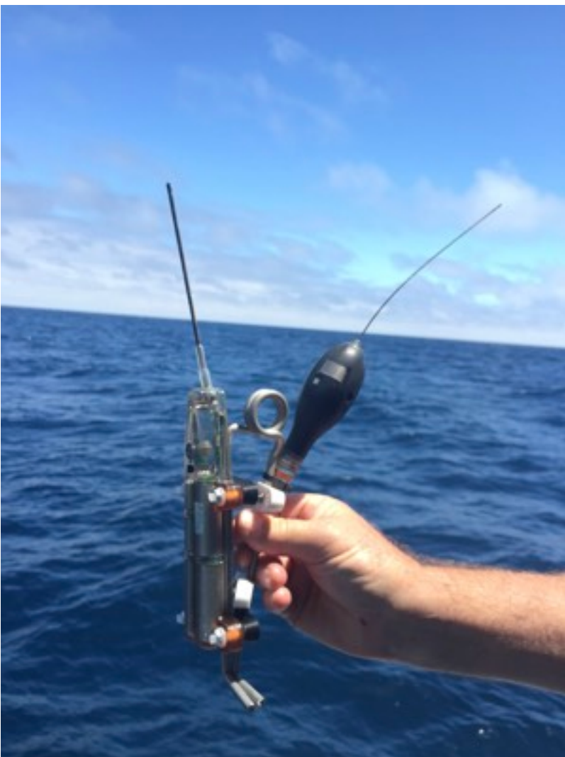
Figure 7: Tags mounted on fin clamps with nylon pads - SPOT6/MiniPAT hybrid tag (Photos ©Sofia M Green, 2020)
