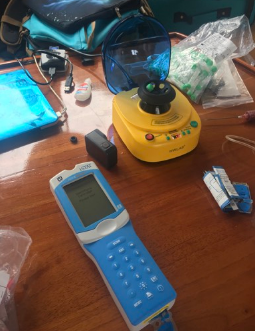
Figure 13: left: i-STAT 300 analyser (which gives blood gas concentrations and lactate acid level) and centrifuge for on board processing and analysis; right: i-STAT results of a female whale shark.
