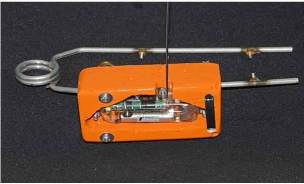
Figure 6. Fin mount SPOT6 prototype previously deployed on juveniles. (Photo: ©Jonathan R. Green 2017).
