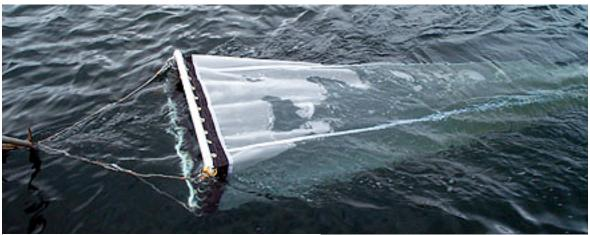
Figure 11. Neuston net for plankton and micro plastic tows
