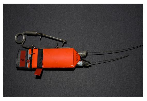
**Figure 6**. CATSCam camera tag with fin bracket, SPOT6 satellite tag and VHF pinger for location and retrieval. (Jonathan R. Green FMME/GWSP/DPNG).
